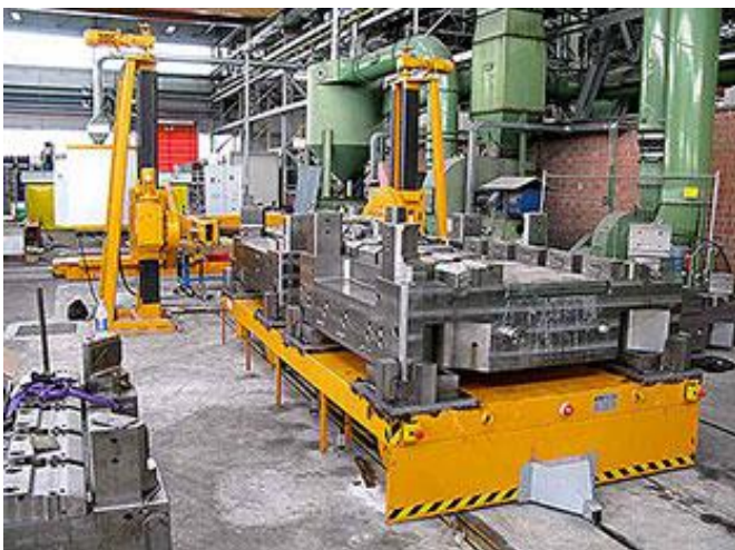
Lift/Rotate Equipment with bespoke mobile carriage.
