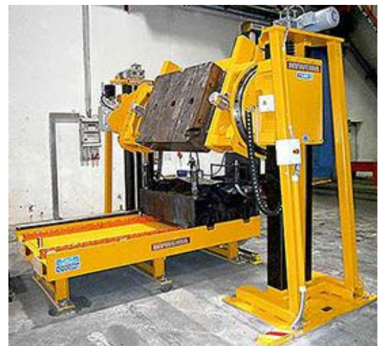
Lift/Rotate Equipment with bespoke fixed to floor carriage.
