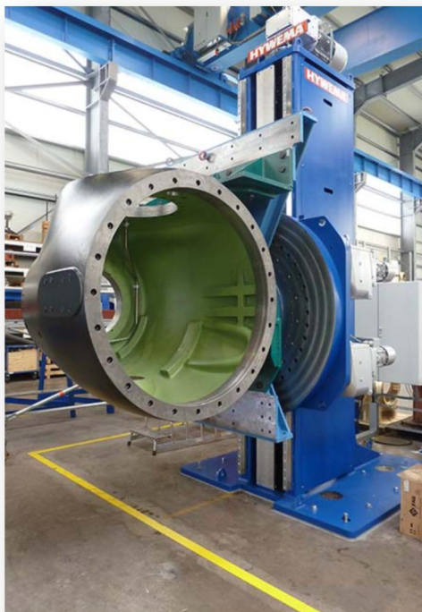
Lift/Rotate Column Max. Capacity: 60 Tons
