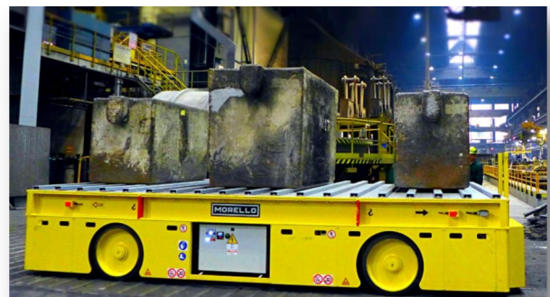
AGV / Motorised Trolley - Platform Max. Capacity: 1000 Tons
