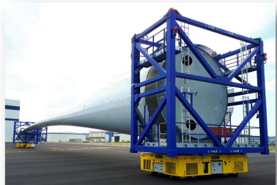
AGV / Motorised Trolley - Platform Max. Capacity: 1000 Tons
